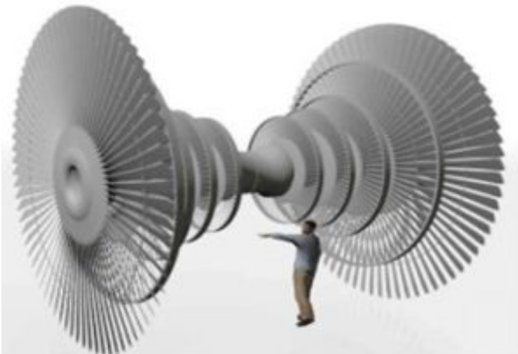
Figure 10.1.a. Steam spins a turbine spins at 3000 rpm—note the person for scale. US DOE, Public Domain.
