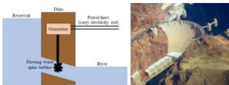
Figure 10.35. Capturing the energy of flowing water. Left (a): diagram of a reservoir created by a dam (in cross section, not to scale); water is directed through a channel to spin a turbine as it flows downstream. Right (b): photo from the downstream side of the Hoover Dam, Nevada, U.S.A.; note the reservoir at upper right. Kelsey, CC BY-NC-SA (a); Licko, Public Domain (b).
