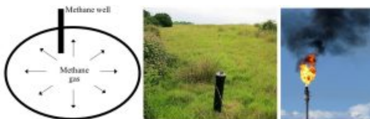
Figure 13.10. Fates of methane generated by anaerobic decomposers in landfills. Simplified diagram of sealed cell with methane well, (cross section, not to scale) left (a); photo of methane well in a capped landfill (approximately 1 meter high), middle (b); photo of a methane flare (they range 5 – 10 meters high), right (c). Kelsey, CC BY-NC-SA. (a); Peter Facey, CC BY-SA (b); W.carter, Pubic Domain (c).
