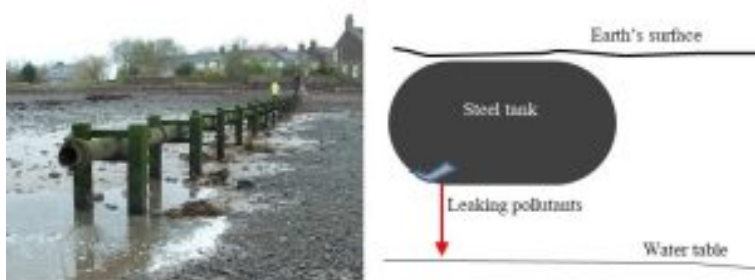
Figure 11.6. Two point sources of water pollution: a pipe releasing sewage into a river, left (a); a diagram of a leaking underground storage tank releasing fuel that could contaminate groundwater, right (b). Right diagram in cross section. John Collins, CC BY-SA (a); Kelsey, CC BY-NC-SA (b).
