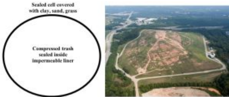
Figure 13.9. Left (a): conceptual diagram of a sealed landfill cell (in cross section—compare to Figure 13.7). Right (b): a landfill made up of many sealed cells. Note the grass growing on top of older cells (aerial photo). Kelsey, CC BY-NC-SA (a); CarlisleEnergy, CC BY-SA (b).
